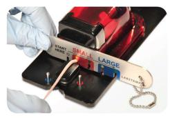
Step 3: Hold the tail across the v-groove, and starting with the smallest slot on the left, to the largest slot on the right of the Tail Gauge, determine the slot that fits the tail. The fit may be snug, but not tight. Do not use force.
