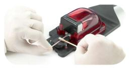
**Step 1:** Apply a thin layer of Tail Oil onto the tail and align the tail within the v-groove of the rubber tail bed.
