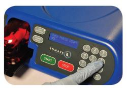
Step 2: Once the Restraint Cartridge STATUS light turns green, enter the desired alphanumeric characters (up to 3) to be tattooed.
