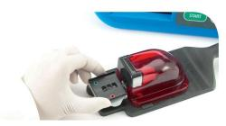
**Step 2:** Align the color-coded Tail Cover holes over the matching alignment posts of the Restraint Cartridge platform, and lower the Tail Cover over the tail allowing the magnets to securely seat it in place.
