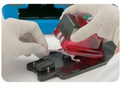
**Step 2:** Pick up a mouse by its tail and place it on the Restraint Cartridge platform. Depress the tail grippers on the red dome cover, position it over the mouse tail, and release grippers.
